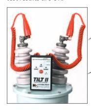
Quick and simple testing of transformers and capacitors for shorts or opens.
