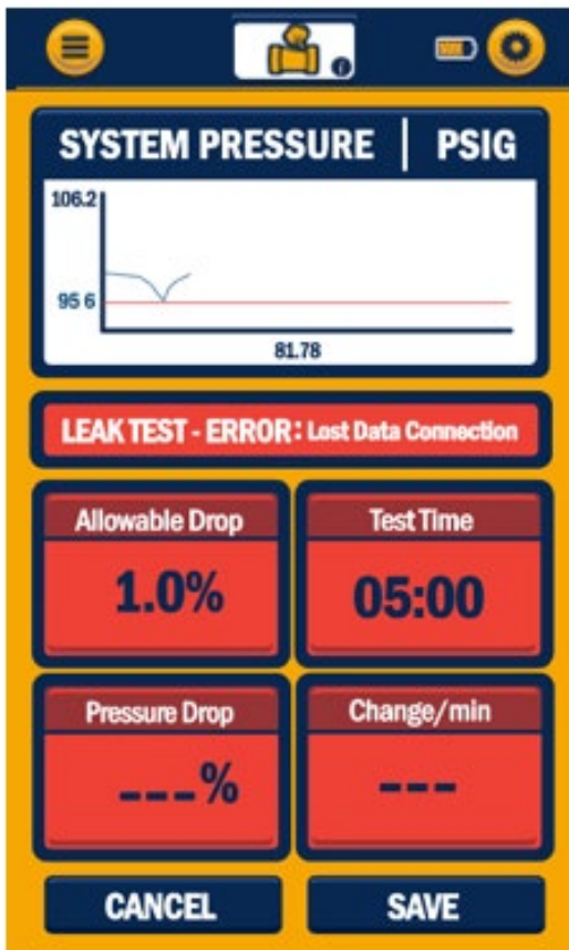
Figure 24: Pressure Decay Test - FAIL
