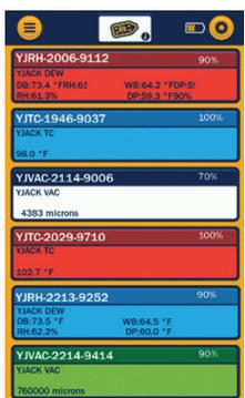
Displays available YJACK® devices to provide data for the sessions the TITANMAX™ connects with the YJACK DEW®, YJACK VAC® and YJACK® Temperature devices. Data is also logged from these devices in the data logging session.
