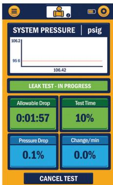
Displays pressure change in the system during a standing pressure test. Allowable Drop is percentage the current system pressure is allowed to drop before the test is deemed a failure. Set the allowable drop percentage.
