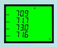
Extech's 12-Channel datalogging thermometer allows for a wide-range of applications with 6 Thermocouple types (J, K, E, T, R,S). It displays CH1 to CH8 or CH9 to CH12 on screen and data can be recorded from all 12 channels simultaneously onto an SD card in Excel® format for further analysis.
