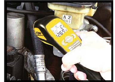
The unit offers simple one-handed operation, laser point sighting, and backlit display feature
