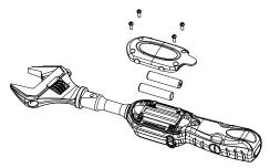
**ATTENTION:** When opening the battery cover of the wrench, you can see a viewing window for the **water contact indicator**. Through this viewing window, you can check if the wrench is damaged by water penetration where the water contact indicator turns red.
