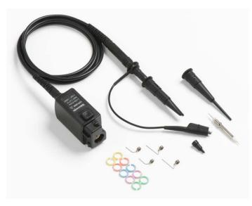
The TPP1000, TPP0500B, TPP0502 and TPP0250 models are high-bandwidth, general-purpose probes from Tektronix that offer breakthrough specifications previously unrealized in this product class. Designed for use with Tektronix MDO3000, MDO4000, MSO/DPO5000, and 5 Series MSO Series oscilloscopes, these probes provide up to 1 GHz of analog bandwidth with less than 3.9 pF of capacitive loading.
