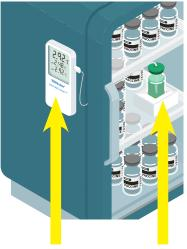
Place data logger on OUTSIDE of refrigerator/freezer Place probe bottle and holder INSIDE of refrigerator/freezer on middle shelf
