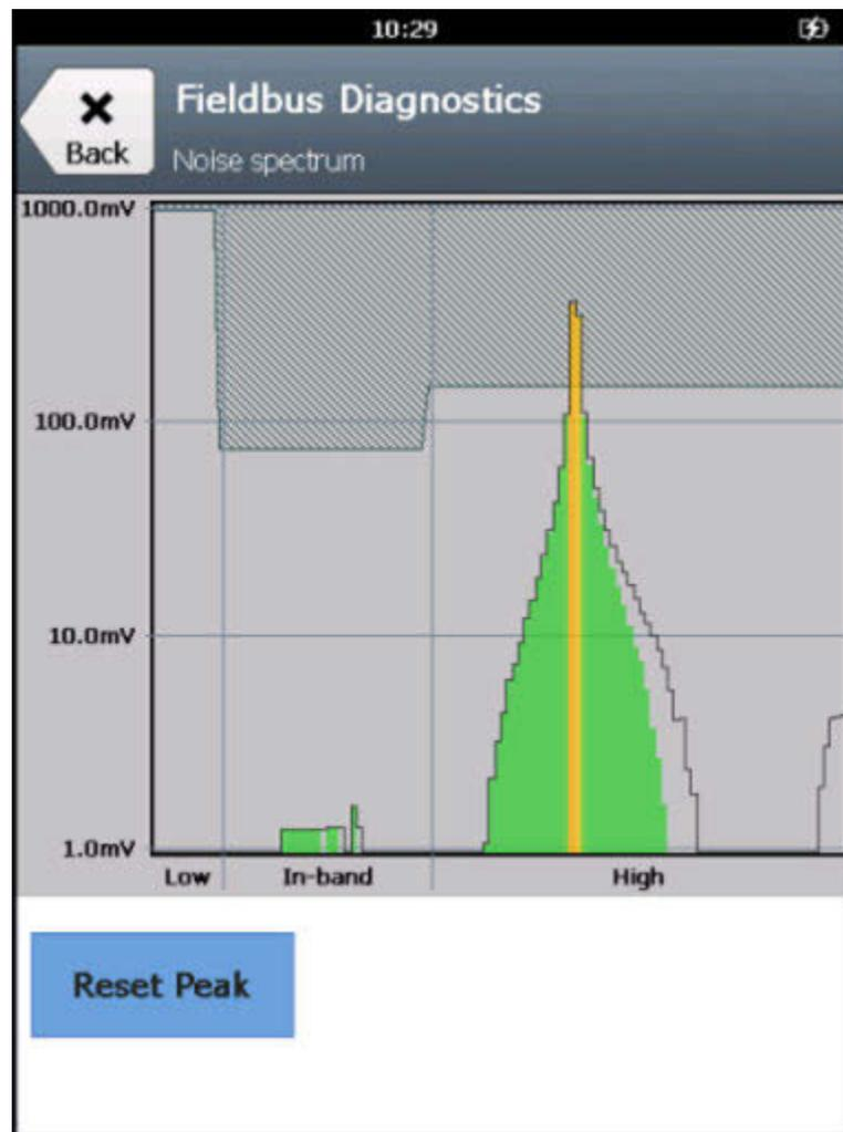
3. If necessary, tap **Reset Peak** to clear the peak on the spectrum.
