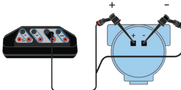
**Figure 3-30: Power a HART positioner**
