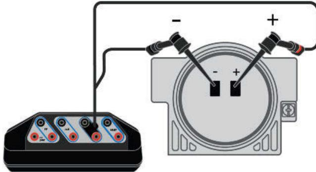
**Figure 4-7: Connect to an externally-powered positioner in-parallel**
