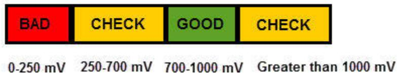
If the fieldbus signal measurement has a BAD or CHECK status, an additional status note is listed on the Fieldbus Diagnostics Overview screen.
