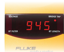
Bridge tap found at 945 feet /288 metres
