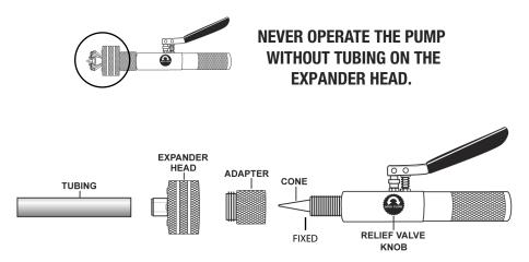
1) Use soft copper tube or heat (anneal) the section of hard copper tubing to be expanded.
