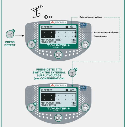
**NOTE**: Once the antenna is aligned using the Detection mode, if it is unknown the channels that can be received at the location, it is advisable to "Auto-Scan" and save the results (see Configuration).
