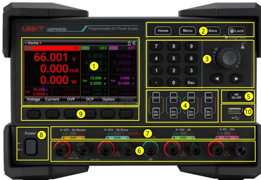
Figure 2-3 UDP4303S Front Panel
