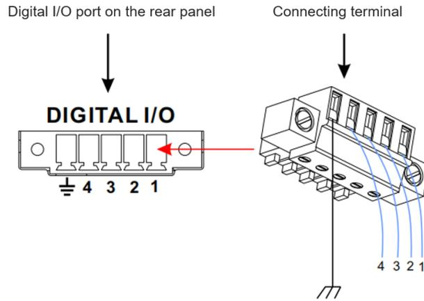
Figure 11-1 Trigger Wiring
