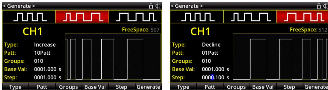
Figure 9-3 Monotonically Increasing Time Template    Figure 9-4 Monotonically Decreasing Time Template
