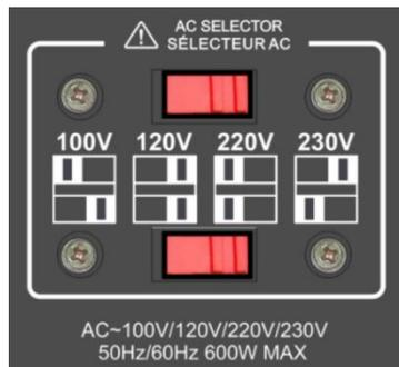
Figure 1-1 AC Selector Switch
