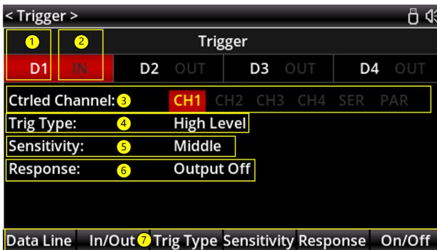
Figure 11-2 Trigger Input
