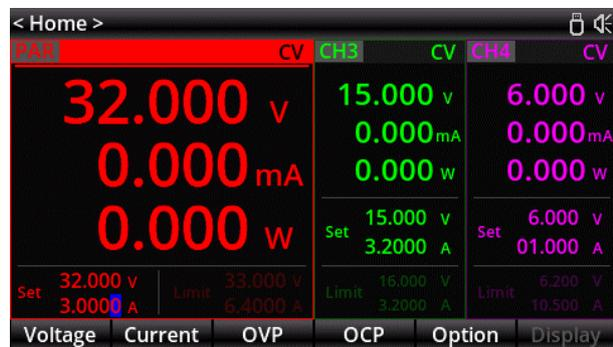
Figure 5-6 Parallel Connection
