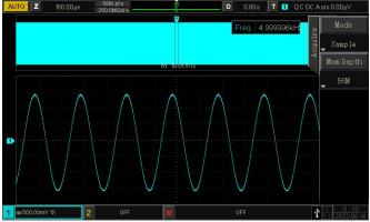
UP01000CS series 56M sampling points per channel. This enables the oscilloscope to maintain high sampling rate in a wider time base range, At the same time considering the whole and details of the waveform, which greatly improves the ability to capture abnormal waveforms.
