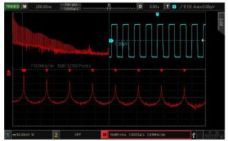
UPO1000CS series has 1 M FFT sampling points. It can also set the practical functions of spectrum analyzer such as frequency range, detection mode and spectrum marking. It is convenient for you to analyze the signal in frequency domain on oscilloscope.
