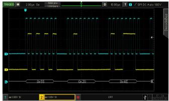
Innovative hardware decoding realizes real-time decoding. The decoding speed with deep storage 56Mpts realizes the millisecond level, which solves the problem of long-time waiting for viewing decoded data. The decoding will not affect the refresh speed of the waveform, and the waveform has the effect of digital fluorescence display. The event list can display the decoded data with deep storage and the time of the packet. These improved technologies will help you better test the serial bus.
