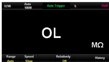
Figure 3-3 Reading of short-circuit test leads
