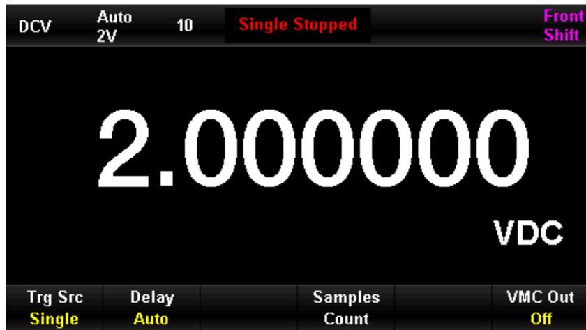
Figure 0-52 Single Trigger Menu
