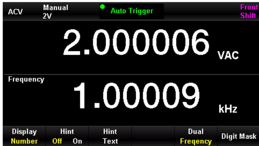
Figure 0-15 Measurement Menu of AC Voltage and Frequency
