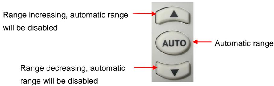
Figure 0-1 Selection Key on the Front Panel
