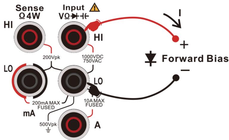
lead to the "Input-HI" terminal and the black test lead to the "Input-LO" terminal.
