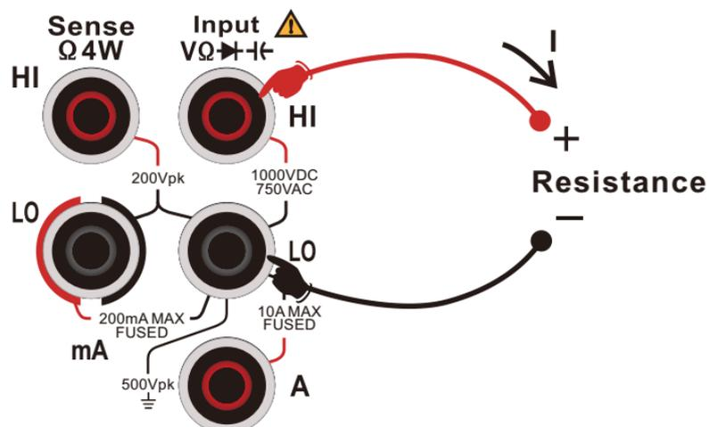
Figure 0-23 Measuring Connection of 2-wire Resistance Measurement
