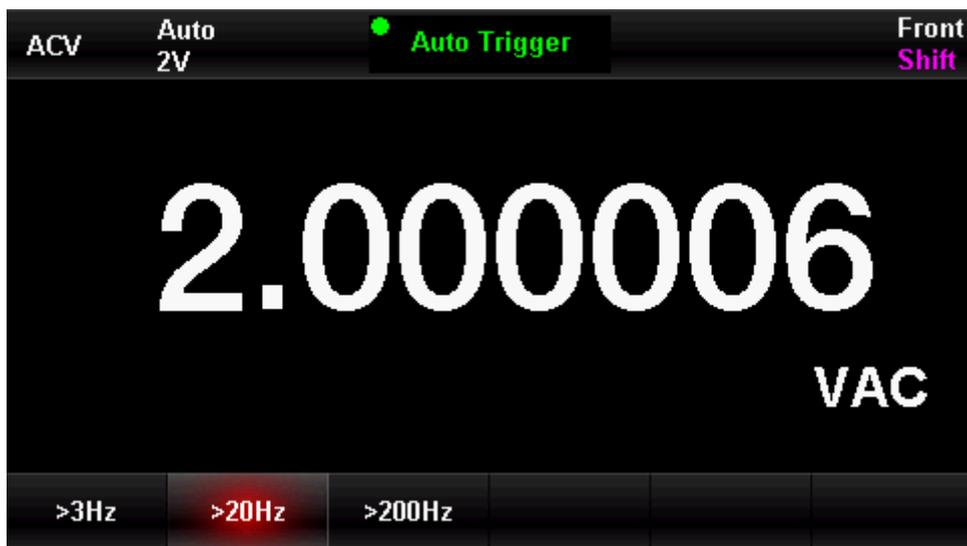
Figure 0-6 Low-frequency Filter Setting
