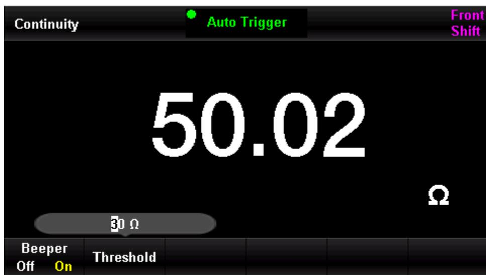
Figure 0-7 Short-circuit Resistance Setting
