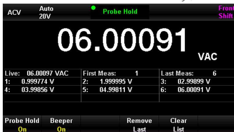
Figure 0-80 ACV Hold Measurement Menu
