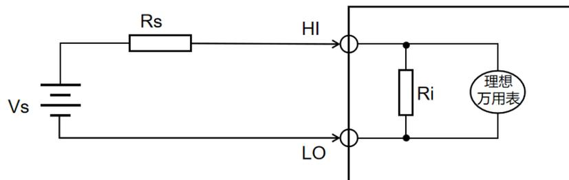
Figure 0-69 Load Error
