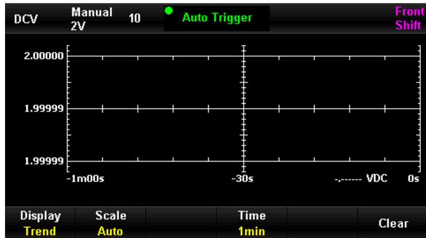
Figure 0-64 Automatic Display in Tendency Mode
