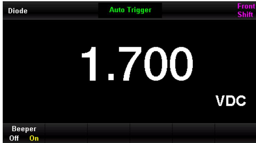
Figure 0-8 Diode Break-over Voltage Measurement
