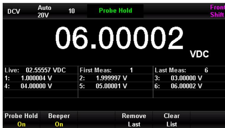
Figure 0-79 DCV Hold Measurement Menu
