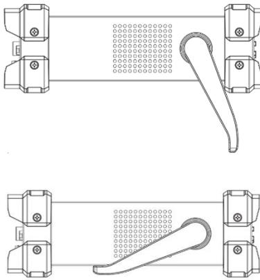
Figure 1-2 Holding Down Position
