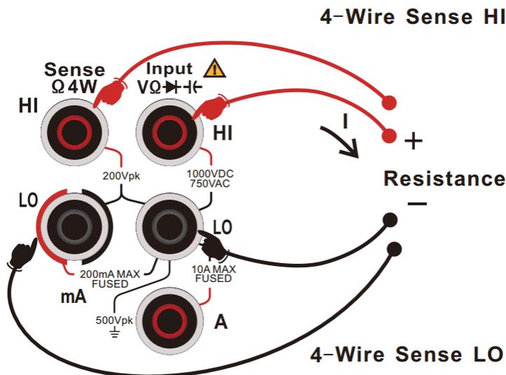
Figure 0-26 Measuring Connection of 4-wire Resistance Measurement
