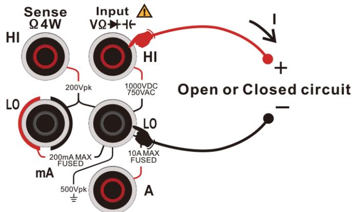
The default value of the short-circuit resistance is  $30\Omega$ , which is set at the factory. The short-circuit resistance can be set by using the arrow keys. The user can directly carry out the continuity test. If the parameter does not need to modify this parameter, it can directly execute the next step.
