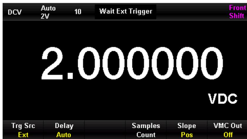
Figure 0-53 External Trigger Menu
