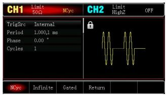
Support pulse string mode: "N cycle", "Gating", "Infinite" Two modulation signal sources: "Internal" and "External".
