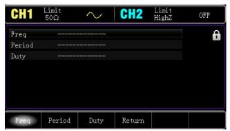
High precision frequency meter, frequency range within 100 mHz~200 MHz can be measured.
