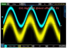
Set small signal superimposed large DC, UTG1000X output noise is lower, with higher SNR.
