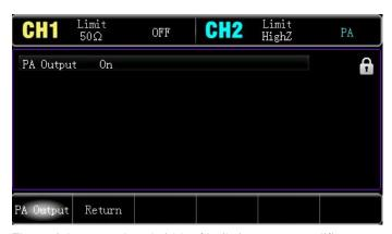
The weight power bandwidth of built-in power amplifier can output up to 100 kHz, the maximum output power 4 W, and output slew rate greater than 18 V/µs.
