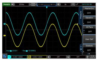
Large output capability at high frequency: 20 Vpp full amplitude output of dual-channel can still be guaranteed at 10 MHz frequency.
