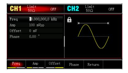
Press Fresoft key to set the frequency, use numerical keyboard to input 10 and then select the unit of
