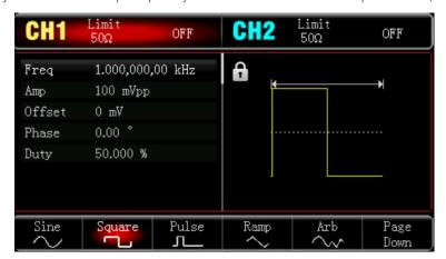
Press Amyoft key to set the amplitude, use numerical keyboard to input 1 and then select the unit of
