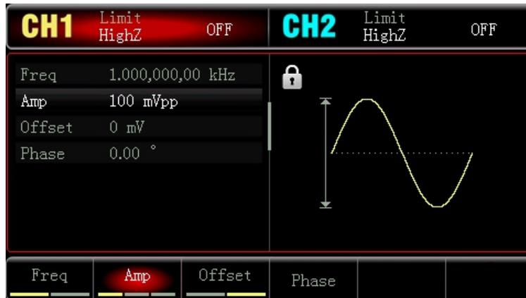
Press **Freq** to set frequency, enter 900 by numeric keypad, and select parameter unit **Hz**.
