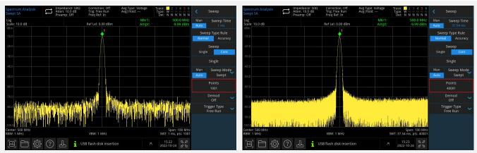
UTS3000A series provides up to 40,001 sweep points, offering higher frequency resolution and making it easier to capture hard-detect signals.
