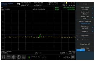
Weak signal testing can be significantly impacted by the noise floor of the spectrum analyzer. With a DANL as low as -165 dBm, UTS3000A series provides excellent sensitivity, enabling effective testing of weak signals.
