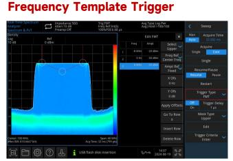
Use the frequency template trigger to generate the measurement of episodic or transient signals.
