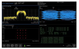
Provides AM, FM, and PM analog signal Analysis; Supports digital signal Analysis for ASK, FSK, PSK, QAM, MSK, DPSK, including EVM calculation.
