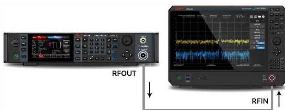
Figure 3-10 Instrument's Setting for Acquiring Single Signal
