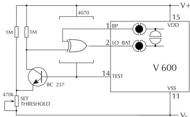
Driving the Battery annunciator with associated external logic and low battery detection circuitry.
