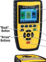
Full-color LCD Display **Function Buttons** perform the function on the display above each button "Test" Button
