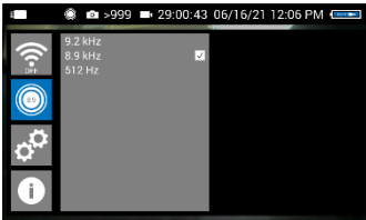
Fig. 32: Locator detection with 8.9 kHz transmission frequency selected
