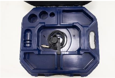
Fig. 61: Monitor cable in the upper shell
