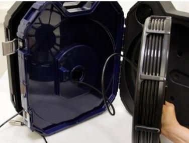
*Fig. 46: Removing the viper with the connection cable from the case.*
