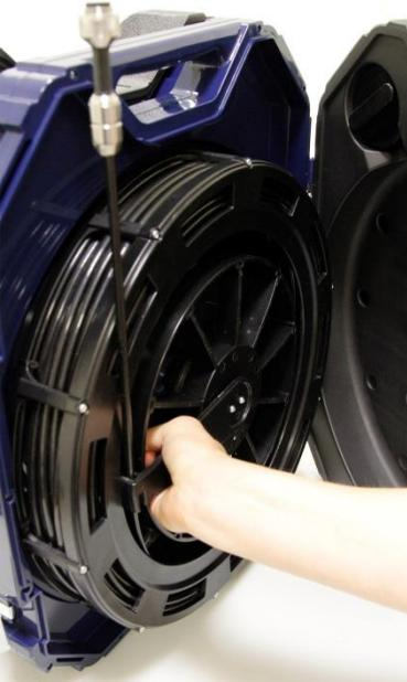
*Fig. 45: Grasping the end of the rod and the viper*
