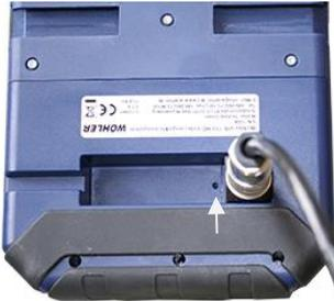
Fig. 40: Reset hole indicated by an arrow
