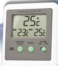
View MIN/MAX readings and set alarms to monitor temperature sensitive materials over any time period
