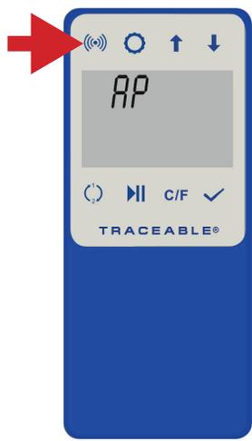
On device Press/HOLD WiFi button for 3 secs. "RP" will appear on display.
