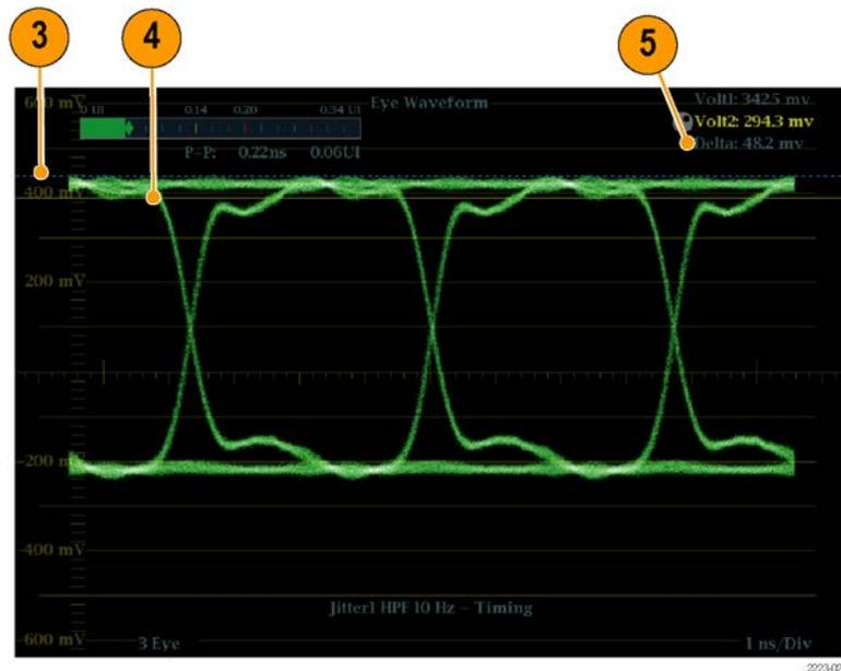
**Figure 56:** Using cursors to measure aberrations in the eye pattern
