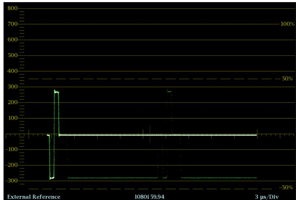
**Figure 23: External Reference Waveform display (tri-level sync signal)**
