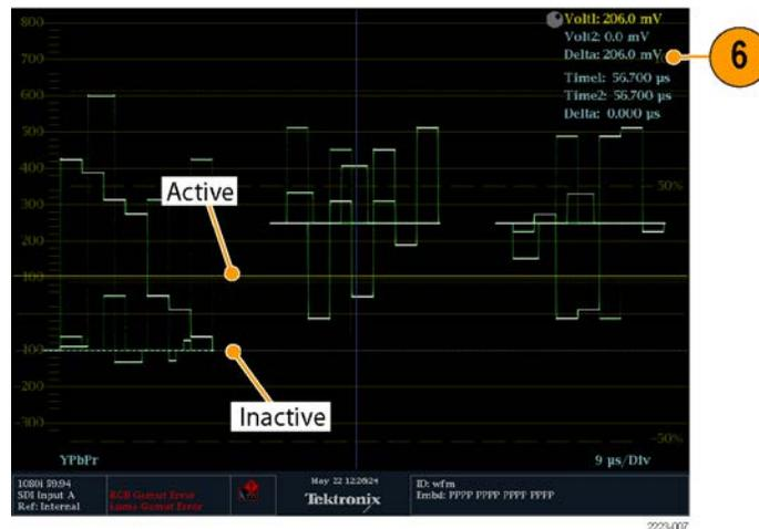
Figure 52: Using measurement cursors in the Waveform display
