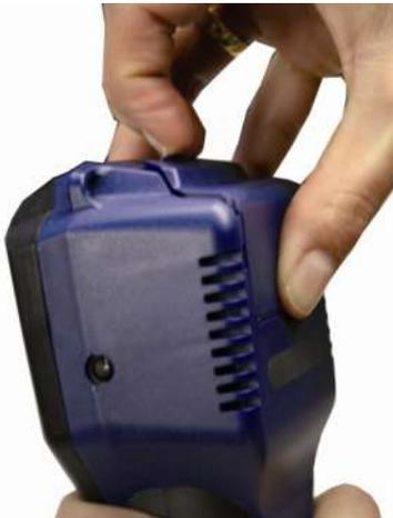
Fig. 10: Open the battery compartment.
