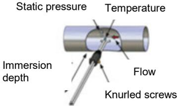
Fig. 19: Measuring the air speed with the S-tube
