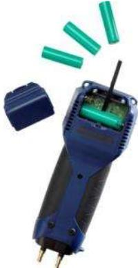
Fig. 9: Position of the batteries in the Wöhler DC 410<sup>FLOW</sup>
