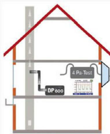
Fig. 42: 4 Pa Test with Wöhler DP 600
