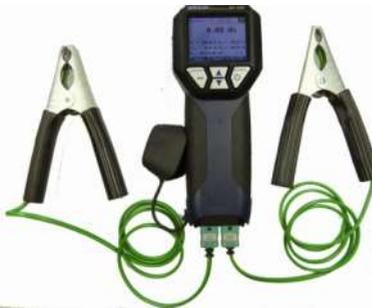
Fig. 4: Connecting a temperature measuring plier
