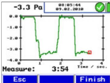
Fig. 40: Pressure profile during the 4 Pa Test
