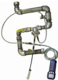
Fig. 55: Volume measurement with the Wöhler DC 410<sup>FLOW</sup> and a syringe (up to 100 ml tube volume).
