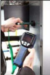
Fig. 53: Application example DC 430<sup>Flow</sup> with Special Wall Temperature Probe
