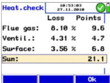
Fig. 52: Evaluation of the Energy Utilization Check
