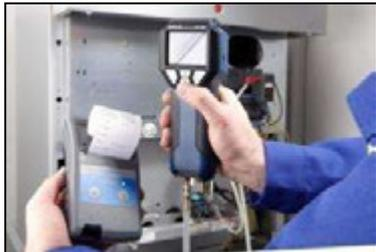
Fig. 60: Transmission of data records from the DC 410<sup>FLOW</sup> to the thermal fast printer TD 600.
