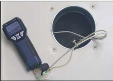
Fig. 31: Example - Connection of the measuring hoses
