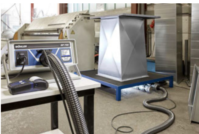
Quality control during series production of ducts and components.
