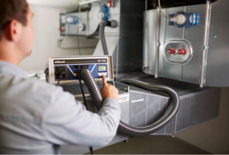
Fig. 11: Example: positive pressure measurement without adapter
