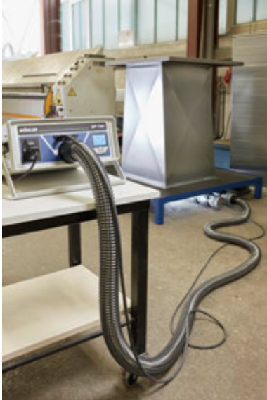
Fig. 12: Example: Measurement according to DIN EN 15727
