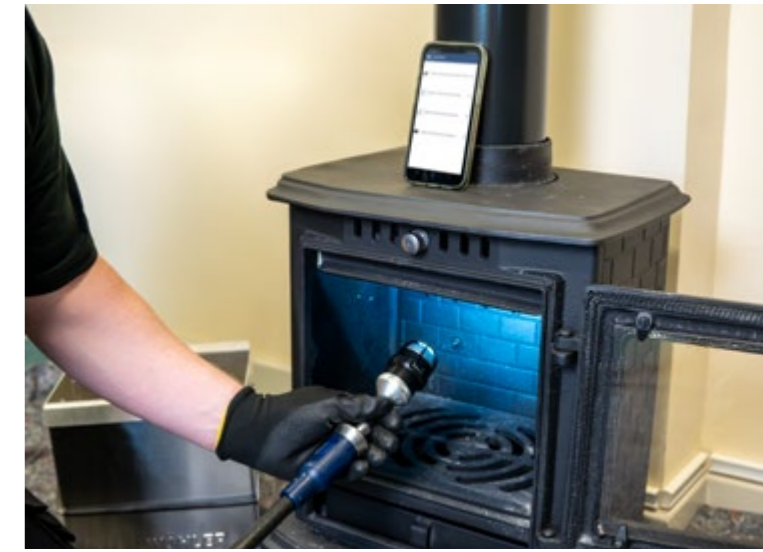
Quickly ready for use: All you need for the inspection is the Wöhler SI 400 Smart Inspection Camera, a suitable viper and your mobile phone
