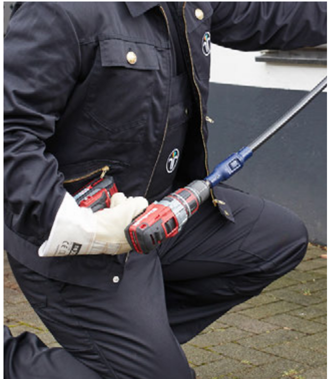
For intensive cleaning, use a cordless screwdriver or drill to rotate the rod.
