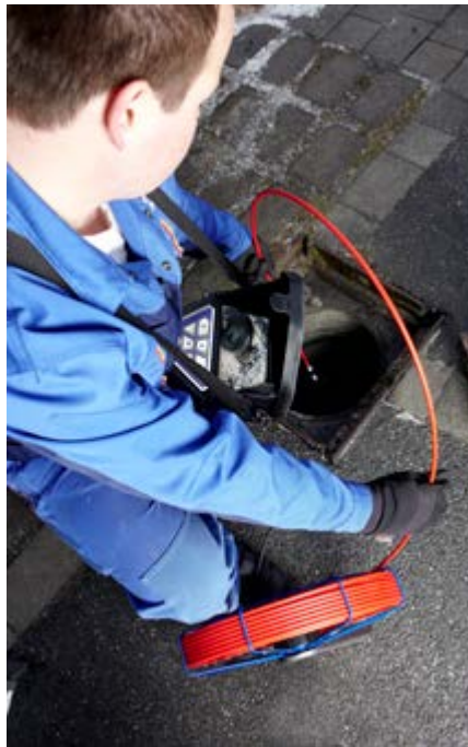
Professionally equipped with camera viper for inspecting underground pipelines.
