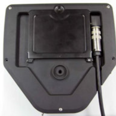
Fig. 9: Camera cable fed through guide
