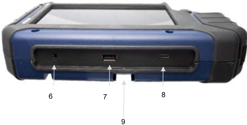
Fig. 8: Monitor bottom with connector strip
