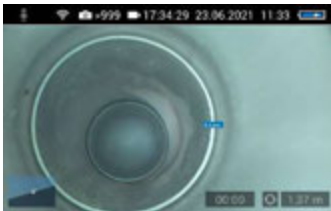
Fig. 25: Focus adjustment , distance is displayed
