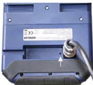
Fig. 67: Reset hole indicated by an arrow
