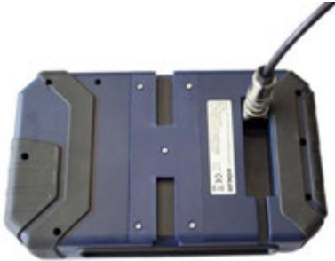
Fig. 10: Camera cable connection
