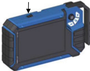
Fig. 17: Push button for pulling out the handle marked with arrow
