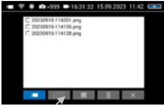
Fig. 36: Image gallery with highlighted files; the Save icon is indicated by an arrow.
