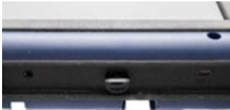
Fig. 9: Insert USB Stick correctly
