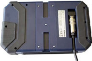
Fig. 11: Camera cable fed through guide
