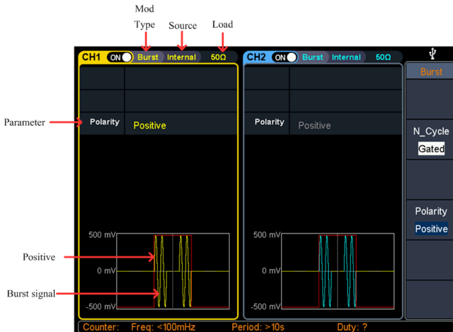
Figure 5-27: Gated burst user interface
