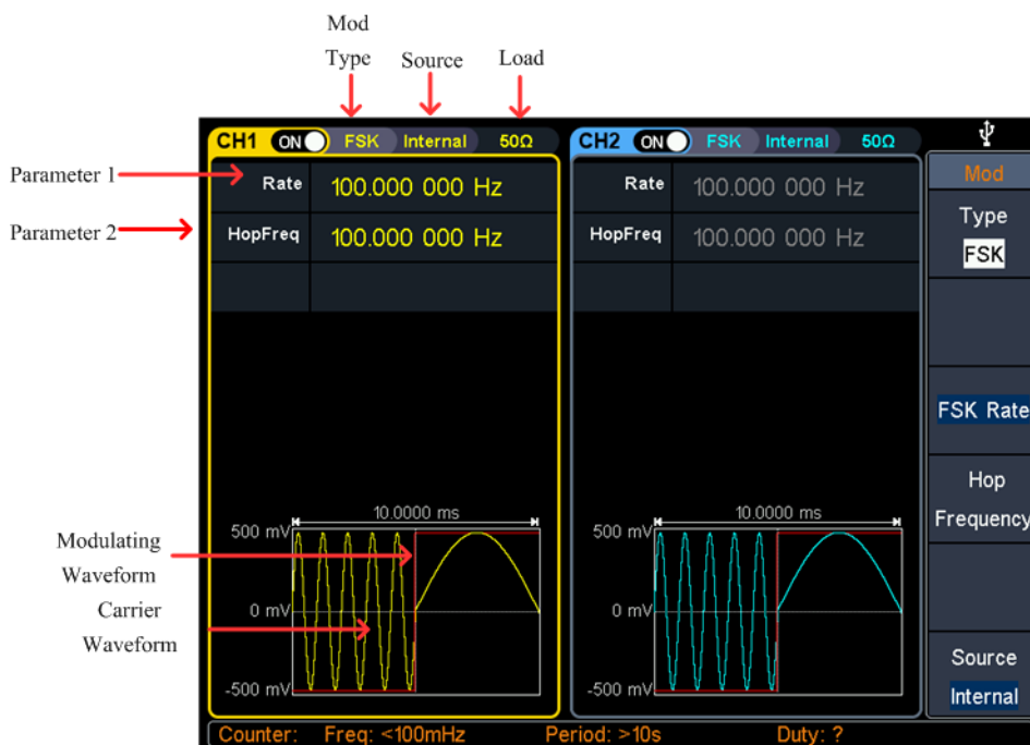
Figure 5-17: FSK user interface
