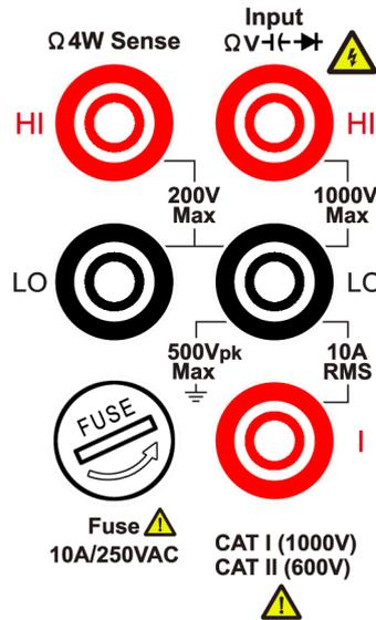
The user-replaceable 10 A current-protection fuse is on the front panel. To maintain protection, replace fuse only with fuse of the specified type and rating. About the specified type and rating of the fuse, please refer to "7 Current Terminal Fuse" in "Front panel overview" on page 7.
