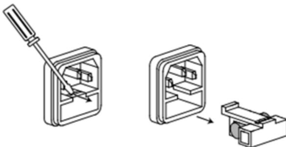
3. Replace the fuse with a new one, which should match with the voltage; install it into the fuse box, and push the fuse box back on to the rear panel.
