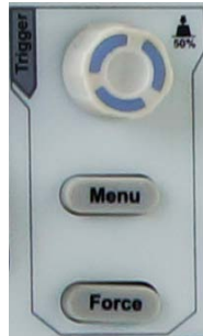
Figure 3-13 Trigger Control Zone
