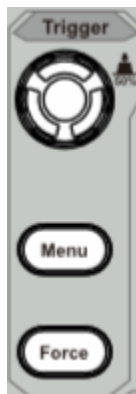
Figure 3-12 Trigger Control Zone
