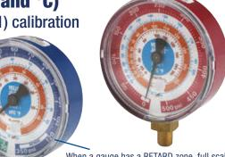
When a gauge has a RETARD zone, full scale is considered to be the last marked reading prior to entering the RETARD zone. For example, this gauge has a full scale reading of 120 psi. Gauge accuracy is not specified in the RETARD zone.
