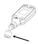
Remove the red plug from the brass quick coupler nut. Then the device can be attached directly to the side port of a core removal tool or to a system service port. A 5/16" adapter (19121 straight or 19221 90 degree) can be used for systems with 5/16" connections. For the most accurate system vacuum readings and to avoid contamination of the sensor, it is not recommended to connect the vacuum gauge directly to the vacuum pump.
