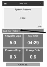
Perform system leak tests and capture test results for service reports.
