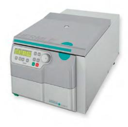
Universal High Speed Centrifuge Z 446 K Max. Speed: 16,000 rpm Max. Volume: 4 x 750 ml Z326-K Refrigerated Centrifuge max. Speed: 18,000 rpm max. Volume: 4 x 145 ml
