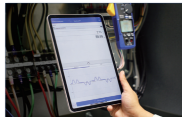
Step 2: Start the app installed to wirelessly connect the terminal with the instrument.
