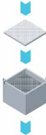
H13 HEPA particle filter and 10% active carbon foam filter
